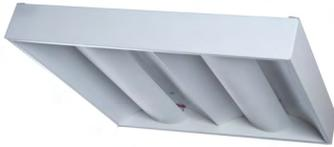
Low profile dedicated to T5 or T8 lamping is ideal for shallow plenum spaces. Specification grade, direct / indirect center diffuser luminaire provides smooth and uniform ambient lighting for all commercial and industrial buildings with recessed configurations. Reflected light from matte surfaces provide a softened "sky light" appearance to the modern office environment. Choice of perforated basket or linear ribbed lens. Recessed perforated dual diffuser with acrylic overlay.
