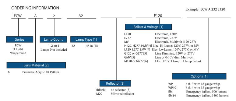
EM14 ballast required for T5 & T5HO lamps
