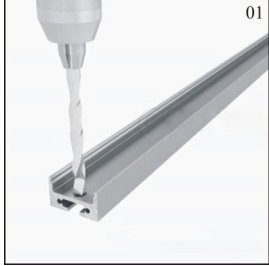
Drill hole for power cord.
