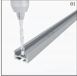
Drill hole for power cord.
