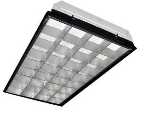
Housing and ends are die-formed from code gauge cold rolled steel. Precision formed anodized semi-specular aluminum louver. Standard normal 3" deep cell louvers are manufactured using interlocked construction and mitred corners. Wiring access plate or knockouts are provided on back of housing for flexible conduit attachment. Ballasts cover and snap into place eliminating the need for tools when accessing the ballast. Listed by and bears *UL* label.
