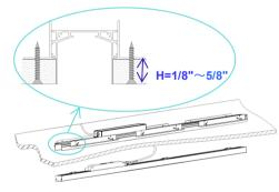
(5) Install 4ft fixture to 4ft Shell
