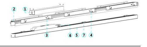
(2) Adjust installation wing to the desired height and secure to the fixture.
