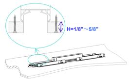
(5) Install 4ft fixture to 4ft Shell
