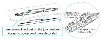
Note: connect to 1, 2, 3 only if do not need to use dimming function, no need to connect 4, 5
