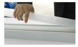
A3. Put carrier uninstallation tool into right position inside of carrier, then pull up
