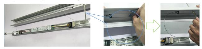
A10. Put one side of carrier on right position inside of main profile, then press carrier
