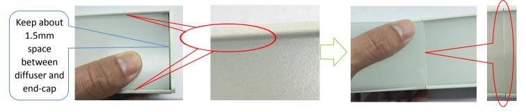
A13. Put anti-lightlead clips in the space between diffuser and end-cap, finish light fixture installation
