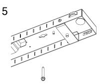
Install EM body to ceiling using desired anchors/ screws (provided by others) 3x
