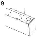
Screw in other end of hanging kit as shown and tighten
