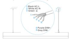
Explain: connect to ①、②、③ only if do not need to use dimming function, no need to connect ④、⑤
